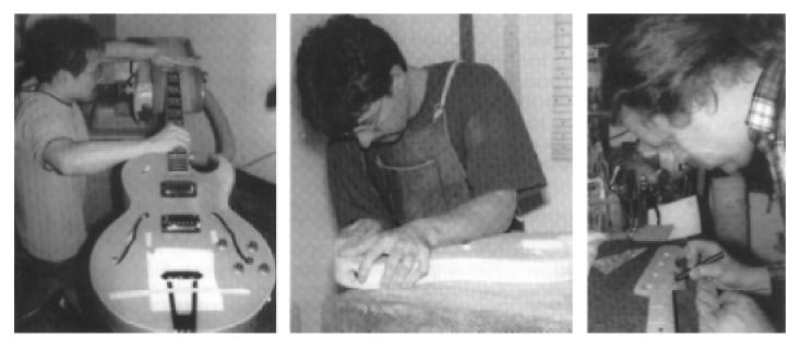
Norio Imai repairing a headstock on a Gibson 175
