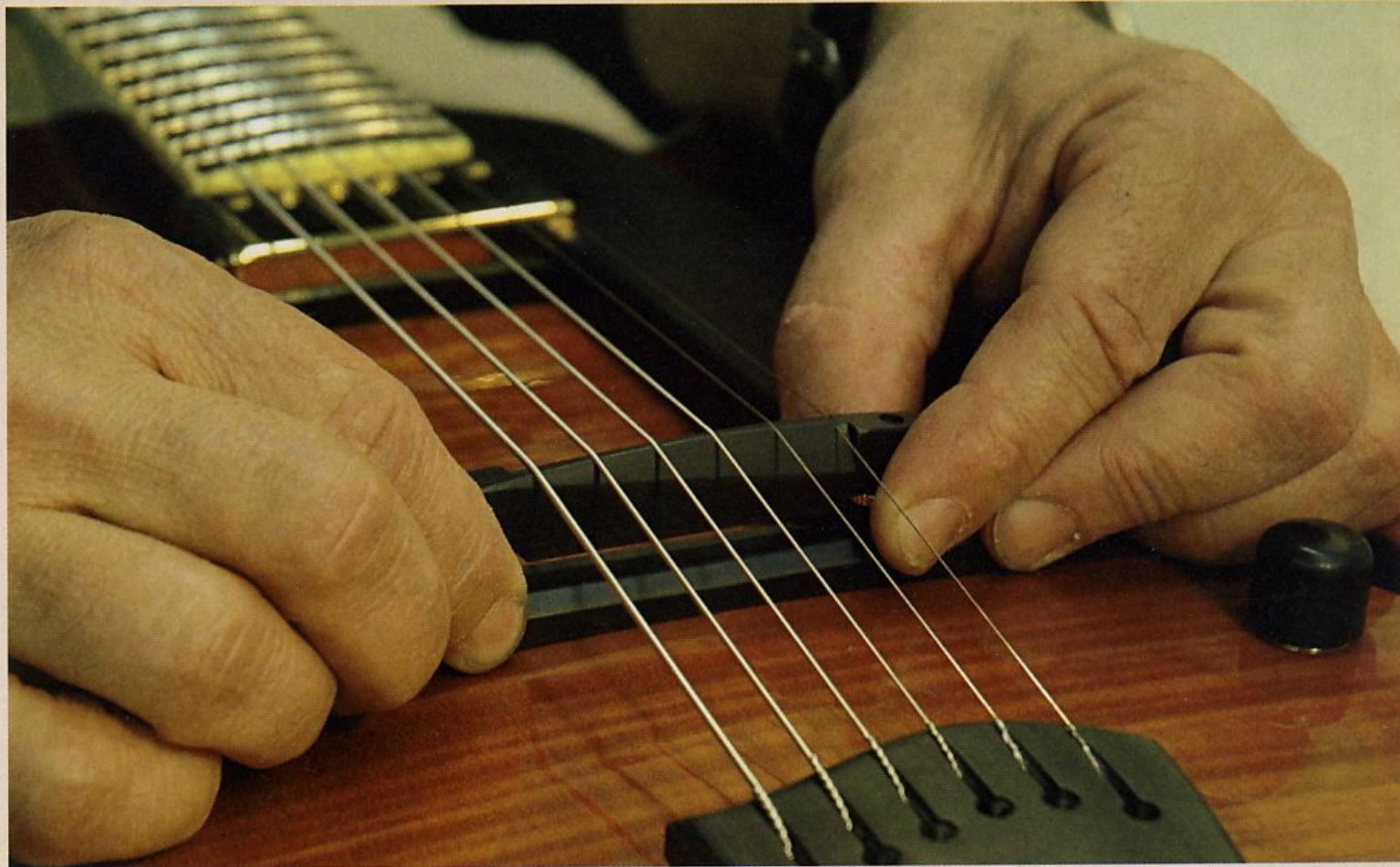
On an archtop with a moveable bridge, precise placement is required for correct intonation and string alignment.
