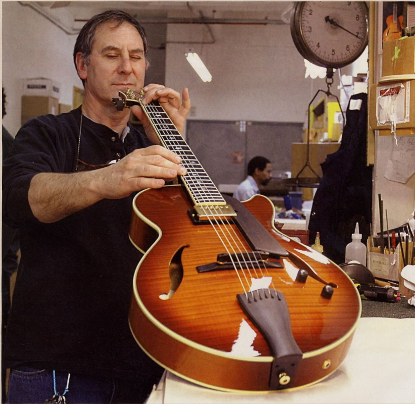
Each Sadowsky archtop gets ten hours of final work and adjustment to assure a flawless setup. Here, Roger Sadowsky checks neck relief by holding the sixth string against the 1st and 14th frets.
